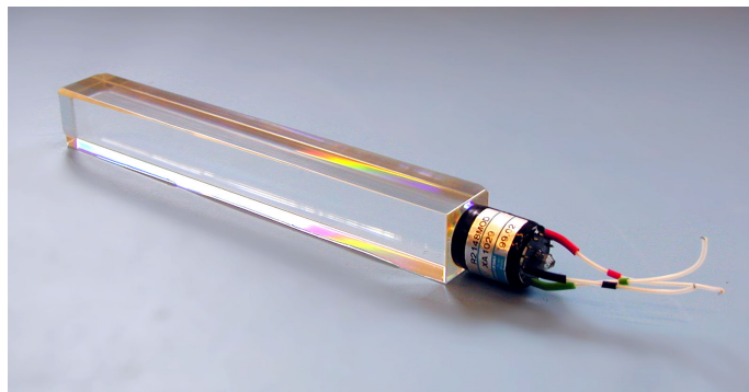
Figure 86: A Crystal of CMS ECAL; its direct connection to the VPT can be observed.
