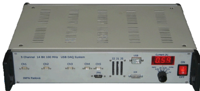
Figure 5.3: Data Acquisition (DAQ) system (INFN of Padova).
