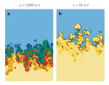
Reactive Rayleigh-Taylor turbulence, showing vertical sections of the temperature field at time t = 128 for two 3D simulations of Rayleigh-Taylor turbulence with different reaction times: (a)  $\tau_r = 1,600 \gg t$  and (b)  $\tau_r = 16 \ll t$ . There is a vertical shift of the mixing layer due to the propagation of the reaction. Images courtesy of N. Vladimirova.
