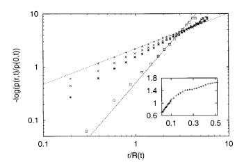
FIG. 4. Right tail of  $-\log(p(r,t)/p(0,t))$  at times t=0.015 (+), t=0.041 (×), t=0.067 (\*), and t=0.77 ( $\Box$ ) in log-log plot. The two lines represent the Richardson slope 2/3 and the Gaussian slope 2. The inset shows the exponent of the right tail of the pdf as a function of time.
