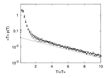
FIG. 7. Pdf of doubling times at resolution N=2048 for distances R = 0.003 (+), R = 0.075 (×), R = 0.02 (\*) and R = 0.046 ( $\Box$ ). The dashed line is the exponential exp $(-0.3T/\langle T \rangle)$ .
