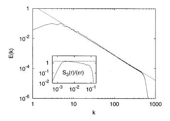
FIG. 1. Energy spectrum E(k) of the inverse cascade simulations at resolution N = 2048 with random forcing around scale  $l_f \approx 0.0074$ . The dashed line is the Kolmogorov spectrum  $E(k) = C\epsilon^{2/3}k^{-5/3}$  with C = 6.0. In the inset it is shown the compensated third-order longitudinal structure function  $S_3(r)/(\epsilon r)$  with the prediction 3/2 (dashed line).
