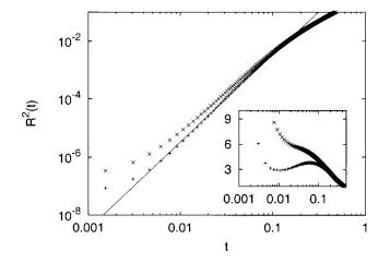
FIG. 2. Relative dispersion  $R^2(t)$  with  $R(0) = \delta x/2(+)$  and  $R(0) = \delta x(\times)$  and the Richardson law  $R^2(t) = g \varepsilon t^3$  with g = 3.8. In the inset the compensated plot  $R^2(t)/(\varepsilon t^3)$  is displayed.
