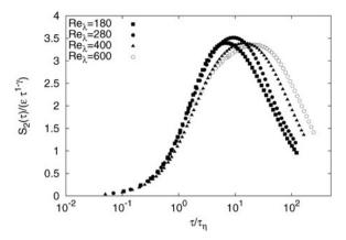
Figure 5. The second-order Lagrangian structure function compensated as  $S_2(\tau)/(\epsilon \tau^{1-\gamma})$ , with  $\gamma = 0.22$ . The anomalous correction  $\gamma$  is extracted from acceleration data shown in Figure (4).
