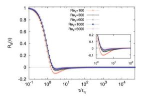
Figure 3. The temporal behaviour of acceleration autocorrelation function  $R_a(\tau) = \langle a(\tau)a(0) \rangle$  derived from the Batchelor parameterisation of the Lagrangian second-order structure function, with exponential large-scale saturation, see Equation (7). Parameters are the same used for Figure 2. In the inset, a zoom in the negative region of the autocorrelation function.
