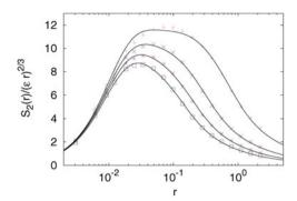
Figure 7. Eulerian second-order structure function  $S_2(r)$  in the inverse energy cascade, compensated with Kolmogorov scaling  $(\varepsilon r)^{2/3}$ . Colours and symbols as in Figure 6. Lines represent the fit with  $(\delta_r u)^2$  as in Equation (13), which gives the ratio  $L/\eta = 12$  ( $\alpha = 0.08$ ),  $L/\eta = 16$  ( $\alpha = 0.06$ ),  $L/\eta = 25$  ( $\alpha = 0.04$ ) and  $L/\eta = 54$  ( $\alpha = 0.02$ ).
