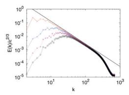
Figure 6. Kinetic energy spectra from 2d direct numerical simulations at resolution  $N^2=2048^2$ , with  $\alpha=0.02$  (red +),  $\alpha=0.04$  (blues ×),  $\alpha=0.06$  (pink \*) and  $\alpha=0.08$  (black  $\square$ ). The line represents Kolmogorov spectrum  $E(k)=C\varepsilon^{2/3}k^{-5/3}$  with C=6.
