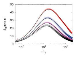
Figure 8. Second-order Lagrangian structure function  $S_2(\tau)$  in the inverse energy cascade, compensated with  $\varepsilon\tau$ . Colours and symbols as in Figure 6. Lines represent the fit with  $(\delta_\tau v)^2$  as in Equation (14), which gives the ratio of times  $T_L/\tau_\eta=7.8$  ( $\alpha=0.08$ ),  $T_L/\tau_\eta=8.9$  ( $\alpha=0.06$ ),  $T_L/\tau_\eta=11.2$  ( $\alpha=0.04$ ) and  $T_L/\tau_\eta=16.1$  ( $\alpha=0.02$ ).
