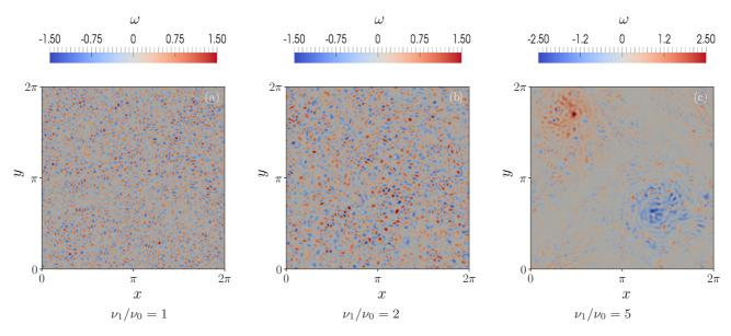
FIG. 3. Visualization of the vorticity field  $\omega(x, y)\hat{z}$  for PCV cases  $v_1/v_0 = 1$  (a),  $v_1/v_0 = 2$  (b), and  $v_1/v_0 = 5$  (c) using samples taken during the statistically stationary state.
