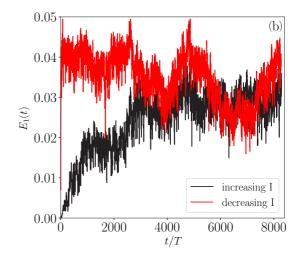
FIG. 8.  $E_1$  as a function of t for run PEV-64-4. The black curve corresponds to flow states obtained by increasing I and the red (gray) curve to flow states obtained by decreasing I. (a) Short evolution times, (b) full time series.
