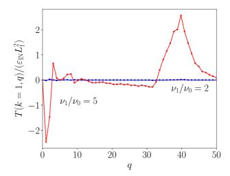
FIG. 10. PCV shell-to-shell transfer function  $T(k, q)/(\varepsilon_{\text{IN}}L_{\text{f}}^2)$  for k=1 and  $1 \leqslant q \leqslant 50$ . Blue (dark gray):  $\nu_1/\nu_0=2$ , without condensate. Red (light gray):  $\nu_1/\nu_0=5$ , with condensate at k=1.
