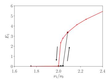
FIG. 5.  $E_1$  as a function of  $\nu_1/\nu_0$ . The black curve corresponds to flow states obtained by increasing  $\nu_1/\nu_0$  and the red (gray) curve to flow states obtained by decreasing  $\nu_1/\nu_0$ . A hysteresis loop is visible in the region  $2.00 \le \nu_1/\nu_0 \le 2.04$ .
