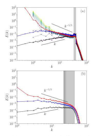
FIG. 9. Energy spectra. (a) PCV with for different values of  $\nu_1/\nu_0$ . The solid lines show the rescaled PCV-B cases  $\nu_1/\nu_0=1$  (black),  $\nu_1/\nu_0=2$  (blue), and  $\nu_1/\nu_0=5$  (red), and the dotted lines PCV-A data. (b) PEV with  $\Gamma_2/\Gamma_0=0.0025$  (red),  $\Gamma_2/\Gamma_0=0.0023$  (blue), and  $\Gamma_2/\Gamma_0=0.002$  (black). The gray-shaded areas indicate the respective driving ranges.
