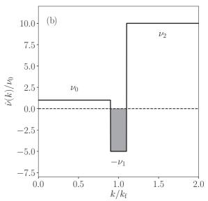
FIG. 1. Effective viscosity for PEV and PCV models. (a) PEV  $\hat{v}/\Gamma_0$  vs  $k/k_{\rm f}$ . (b) PCV  $\hat{v}(k)/v_0$  vs  $k/k_{\rm f}$ . The gray-shaded area corresponds to the interval  $[k_{\rm min}, k_{\rm max}]$ , where the amplification occurs.
