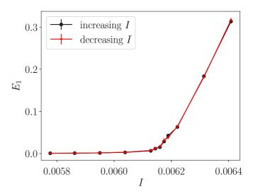
FIG. 7.  $E_1$  as a function of I for series PEV-64. The black curve corresponds to flow states obtained by increasing I and the red (gray) curve to flow states obtained by decreasing I.
