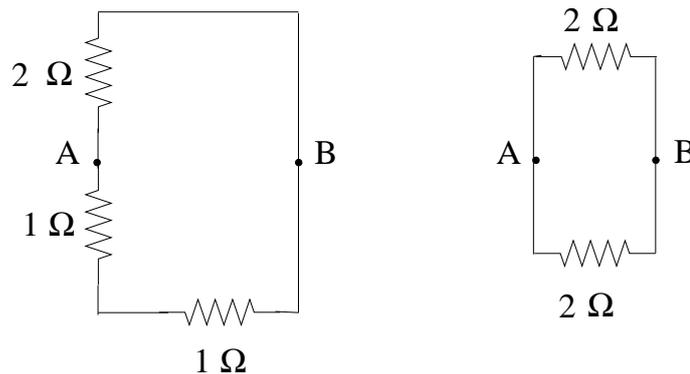
$$I_R = V_{Th}/(R + R_{Th}) = -3/3 = -1 \text{ A}$$
