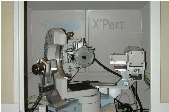
X-Ray diffraction: crystal quality + composition
