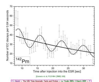
Fit parameters of <sup>140</sup><sub>59</sub>Pr data  $N_0\lambda_{EC}$  $\chi^2/DoF$ 34.9(18) 0.00138(10) 107.2/73 35.4(18) 0.00147(10) 0.18(3) 0.89(1) 67.18/70 Fit parameters of  $^{142}_{61}$ Pm data  $N_0\lambda_{EC}$  $\chi^2/DoF$ 0.0240(42) 46.8(40) 63.77/38
