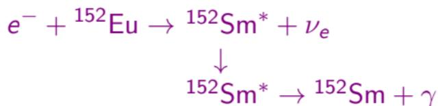
The neutrino helicity is the same as the measurable helicity of the photon when it is emitted in the same direction of the  ${}^{152}\text{Sm}^*$  recoil.
