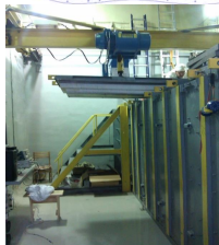
Passive shielding - 60 tons
