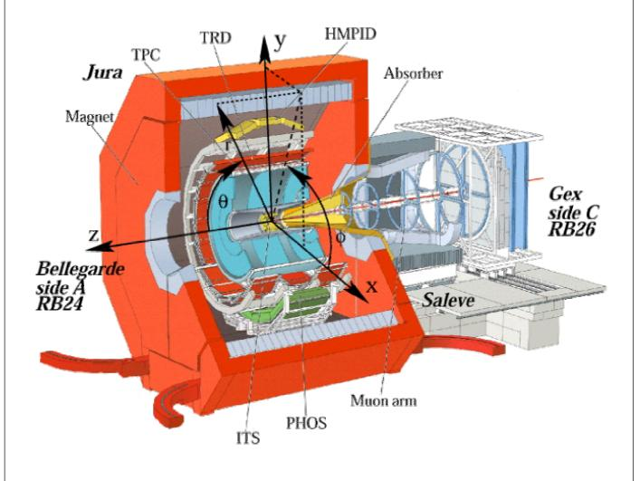
Fig1. Definition of the ALICE coordinate system axis, angles and detector sides.
