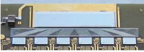
Fig. 3. The 384-strip detector together with the pitch adapter and 6 RX64DTH ASICs.
